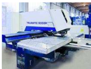
Stanzmaschine 16t, 25t, 45t
