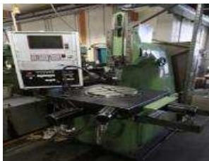
Vertikal Stossmaschine Hub max = 700mm
