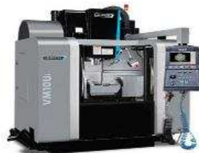
CNC 5-Achs-Maschinen Hurco VM10Ui X-max: 530 mm Y-max: 405 mm Z-max: 480 mm A = -110^{\circ}/+30^{\circ} , C = 360^{\circ}
