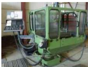
Universal Fräsmaschine Xmax = 1.500 mm Ymax = 500 mm Zmax = 800 mm
