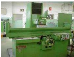
Planschleifmaschine Xmax = 600mm Ymax = 250mm Zmax = 400mm
