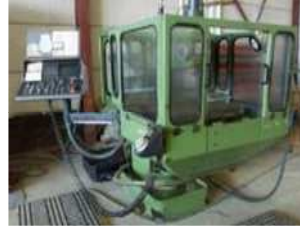
Universal Fräsmaschine Xmax = 1.500 mm Ymax = 500 mm Zmax = 800 mm
