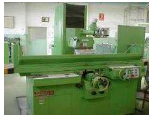
Planschleifmaschine Xmax = 600mm Ymax = 250mm Zmax = 400mm
