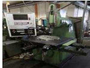
Vertikal Stossmaschine Hub max = 700mm
